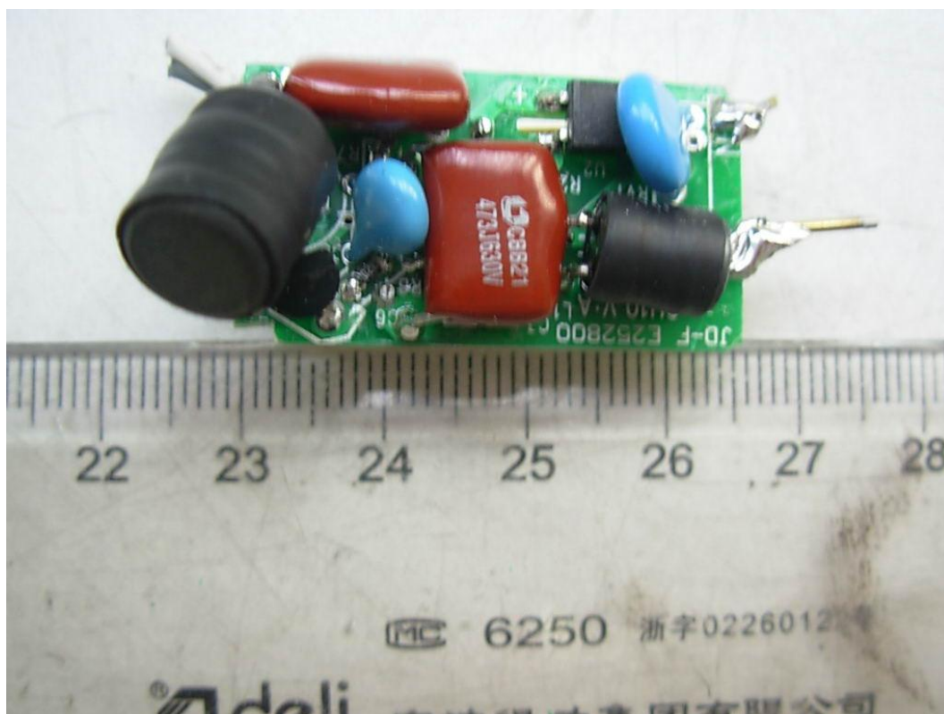
FIGURE 12. LED SPOT LIGHT (M/N: 50-45EUS) MAIN BOARD (SOLDERED VIEW)
