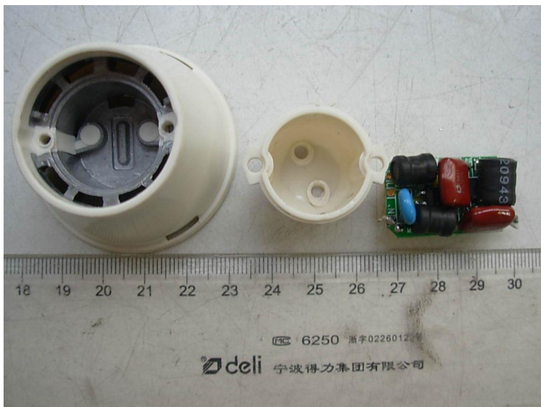
FIGURE 4. LED SPOT LIGHT (M/N: 50-45GUS) MAIN BOARD REMOVED
