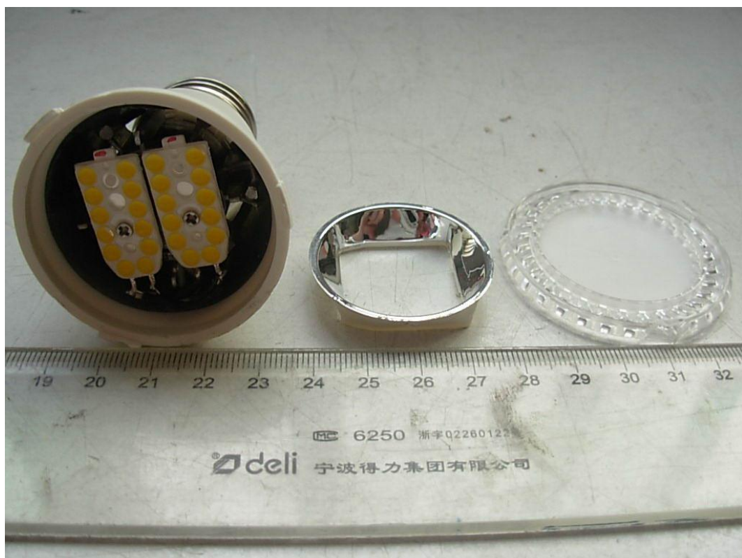
FIGURE 8. LED SPOT LIGHT (M/N: 50-45EUS) COVER REMOVED
